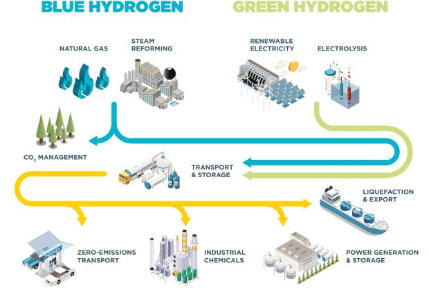
Electrolysis is a process that splits hydrogen from water using an electric current, which does not release GHG emissions. Hydrogen produced through electrolysis is referred to as 'green hydrogen' only when the production is powered by renewable energy.
