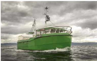
The first diesel-battery fishing vessel (2016)
